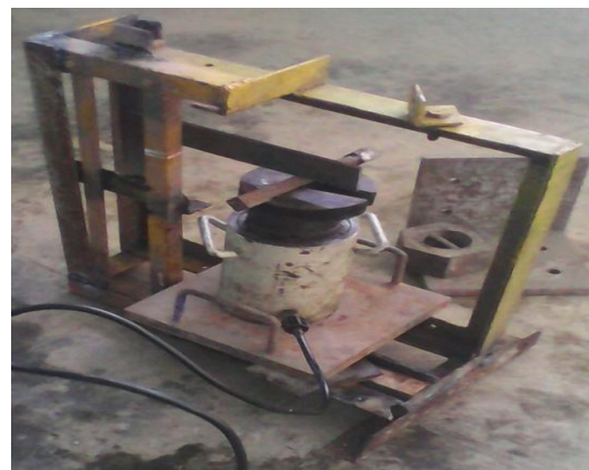
Fig 2.2 Mounting & Loading of Test specimen
