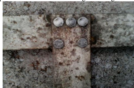
Fig 3.1 Test Specimen of Unsymmetrical bolted joint
